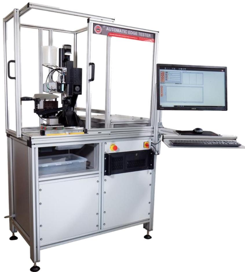
**CATRA has been involved in the testing of performance characteristics of blades for over 50 years.** In particular, the problems of evaluating the cutting ability have been studied using various manual and mechanical methods. This knowledge has enabled CATRA to design an automatic test machine that meets the requirements of consumers, manufacturers and the ISO 8442:5 Standard.
