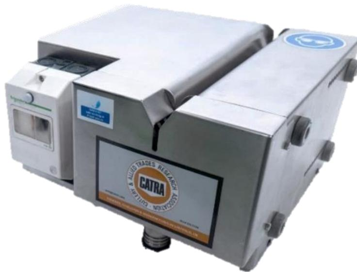
The i-100 operates using the Spiral Interlock Grinding Wheel system known throughout the world of knife manufacturing and sharpening, and one that CATRA has been using for over 40 years. By coupling this system with the high-tech abrasive Cubic Boron Nitride (CBN), it provides CATRA knife sharpeners with many advantages.
